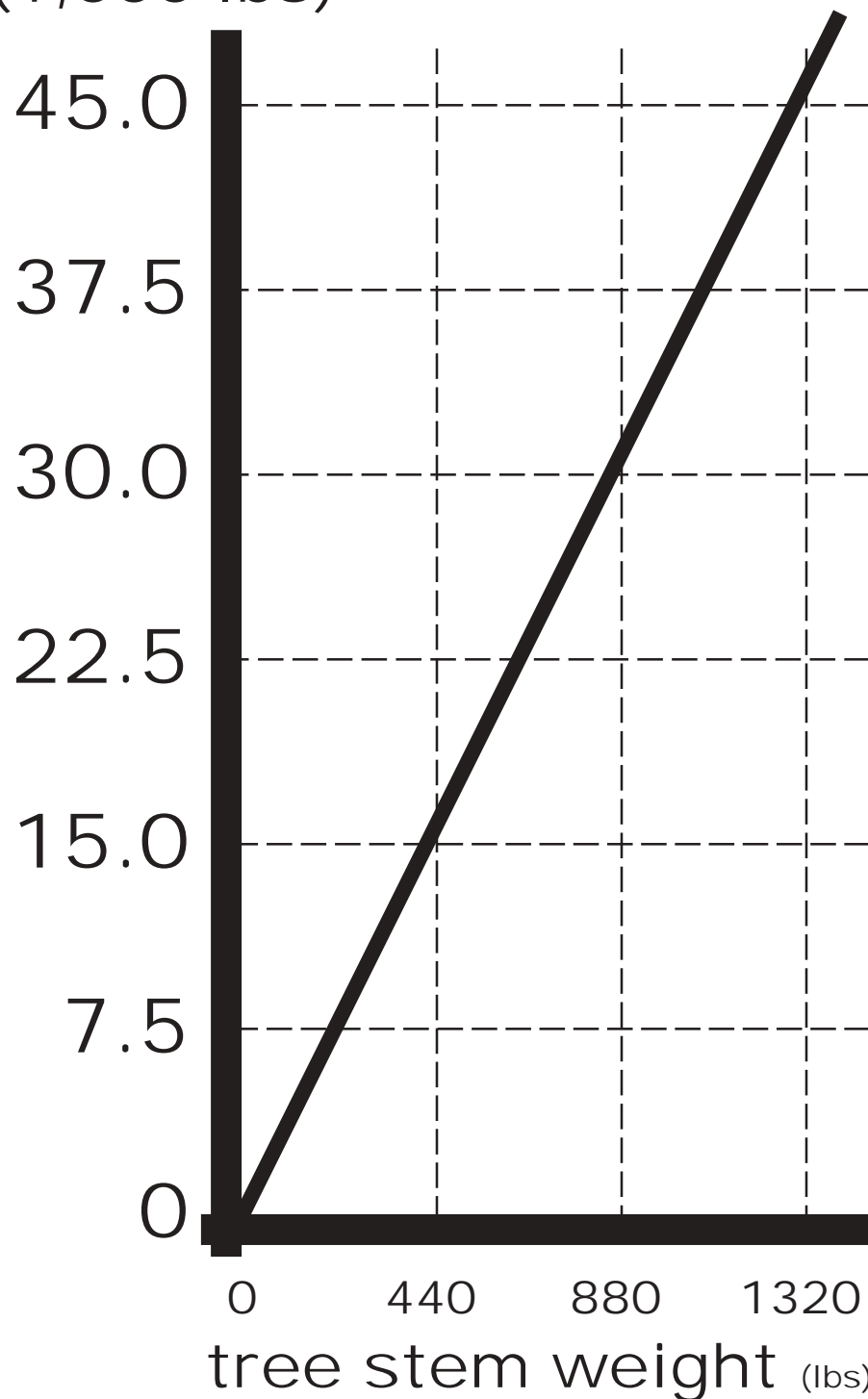
Figure 7: Critical turning force in 1,000 of pounds needed for a given stem weight in pounds. For spruce and fir on different sites. (modified from Achim et al. 2005)
